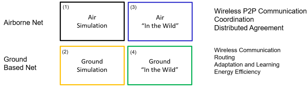
Figure 1: The methodology of the GrADyS Project, illustrating its 4 simulation components in the laboratory and in the field (a.k.a. in the wild).
