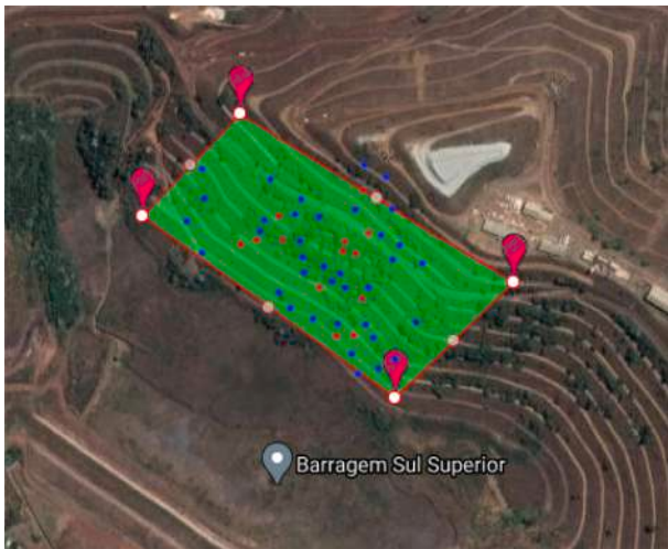
Fig. 5. The same random map with 50 nodes, spread across a similar 105,000 sqm area — a high-risk tailings dam located in Barão de Cocais, MG (Brazil). 9
